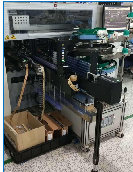
Mirae odd form machine install tube feeder+bowl feeder+radial tape feeder
