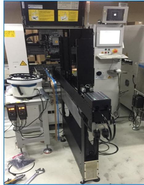
JUKI odd form machine install tube feeder+bowl feeder+radial tape feeder
