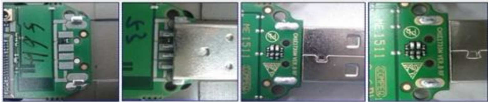
Solder joints formed after furnace
