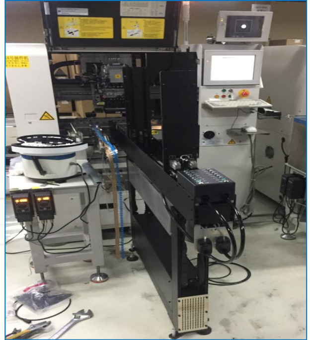
JUKI odd form machine install tube feeder+bowl feeder+radial tape feeder
