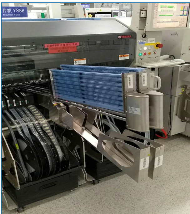
YAMAHA odd form machine install tube feeder
