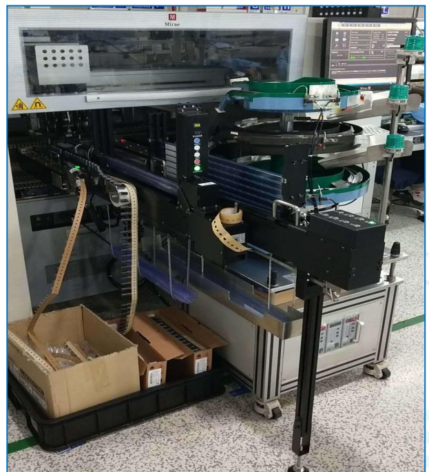
Mirae odd form machine install tube feeder+bowl feeder+radial tape feeder
