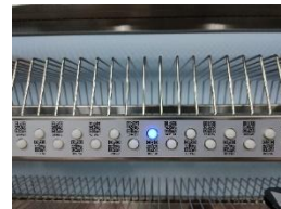
The empty position lights up, prompting to put materials
