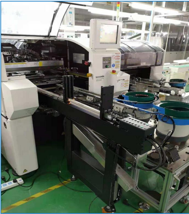
Panasonic CM602 odd form machine install tube feeder+bowl feeder
