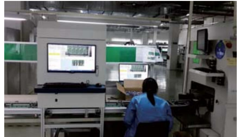
AVI online checking before wave solder
