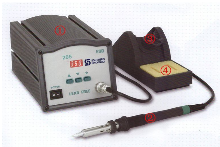
① main engine + ② handle + ③ iron Stan + ④ clean-sponge
