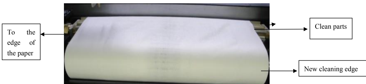
Figure 7-2 Cleaning paper installation
