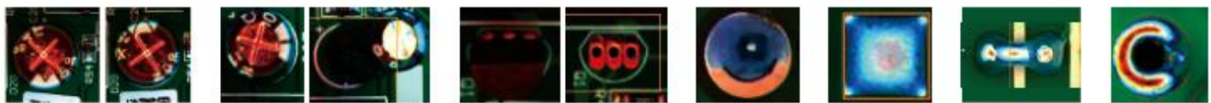
▲ Good ▲ direction ▲ good ▲ deviation ▲ good ▲ missing ▲ tin hole ▲ no foot ▲ tin ▲ missing needle
