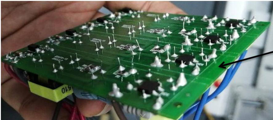
Requires PCB have a process edges, to fix the PCB and facilitate machine operation
