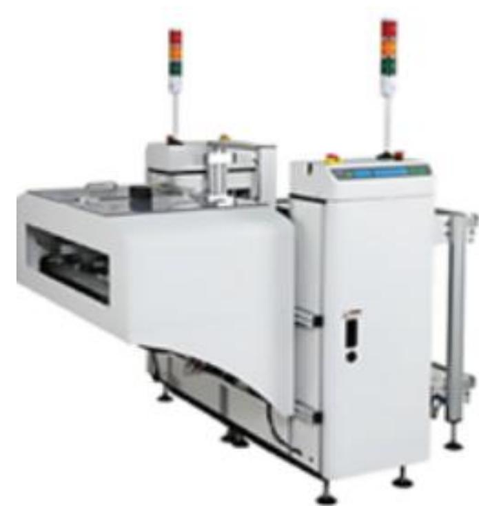
***The unit loads your dual-track production line automatically by pushing PCB's out of a magazine onto the conveyor of the downstream machine.***
