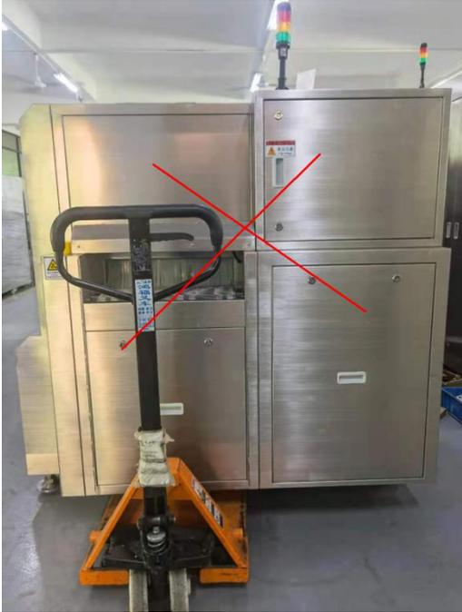
DO not lift the machine from PCBA input side and PCBA output side when you moving the machine.
