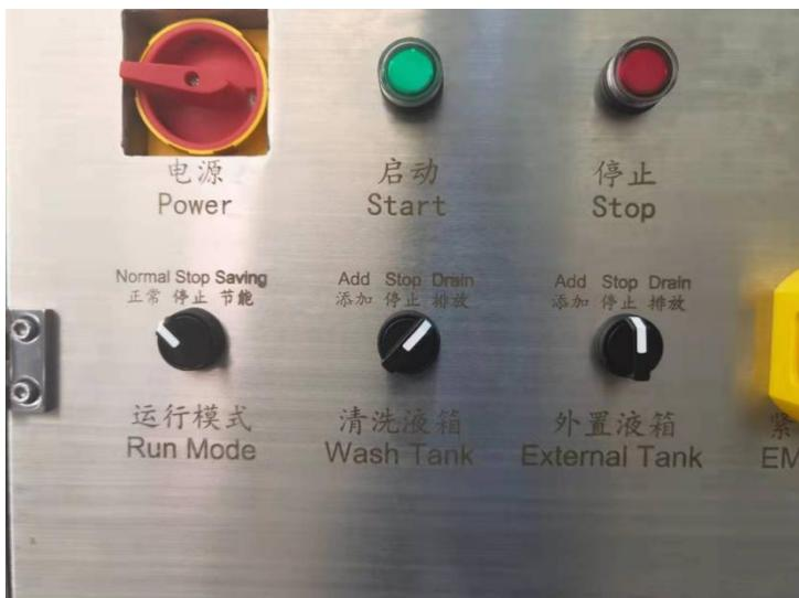
5) Turn on the diluent liquid discharge valve slowly. Liquid will absorb from wash tank to container, flow direction: wash tank--electric diaphragm pump--liquid discharge hose--out side containers(barrels). Please prepare several containers for the waste liquid and do it one by one. If you change container, pls turn off the discharge manual valve off temporary and turn it on again when you replaced new container.
