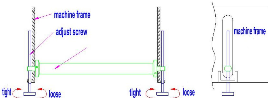
Figure 8-10 net tension adjustment
