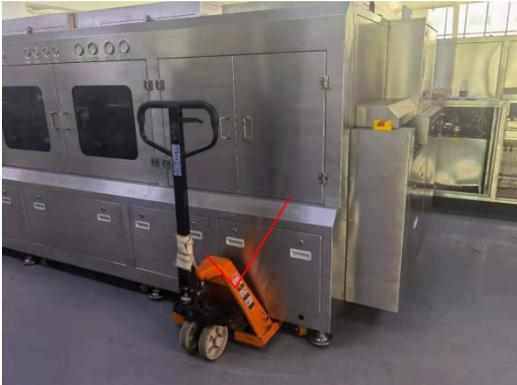
Please lift it from machine front side or rear side when you moving the machine.
