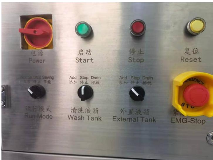
6) Turn on the concentrate liquid add valve slowly. Concentrate liquid will absorb to external tank. Liquid flow direction: outside container-- concentrate liquid add hose--diaphragm pump--concentrate liquid add extension hose--external tank.
