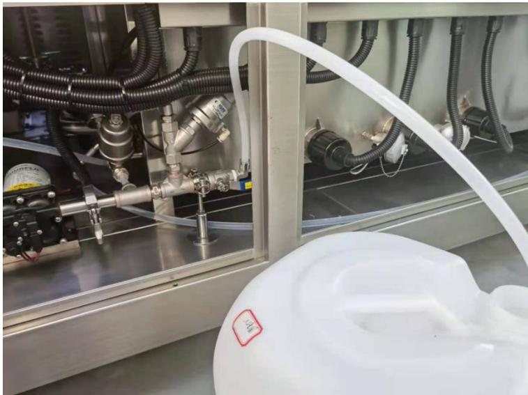
**(Caution: Please hold the hose firmly to avoid the liquid spray out and watch to turn the manual off slowly when one container is going to full.)**
