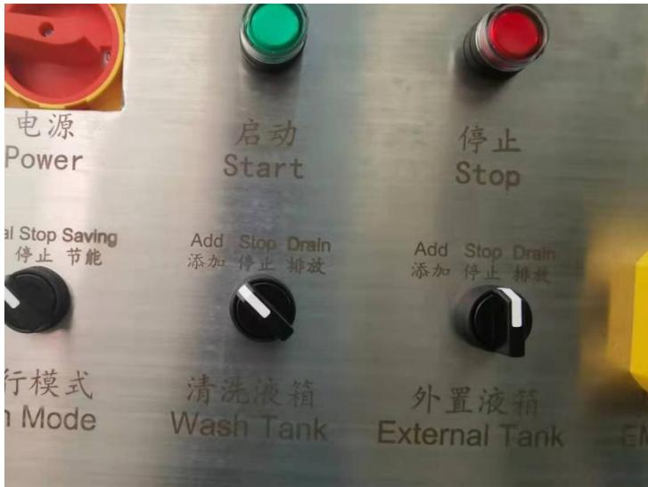
6) Turn on the diluent liquid add valve slowly. Liquid will absorb to wash tank. Diluent liquid flow direction: outside container-- diluent liquid add hose--diaphragm pump--diluent liquid add extension hose--wash tank.
