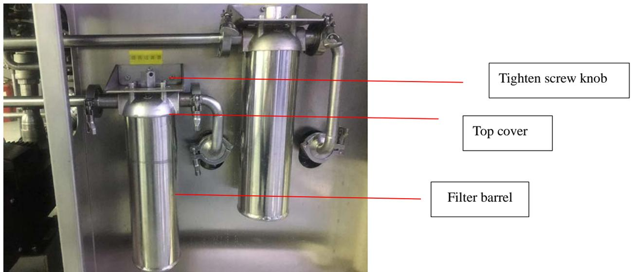
Picture 1 filter barrel
