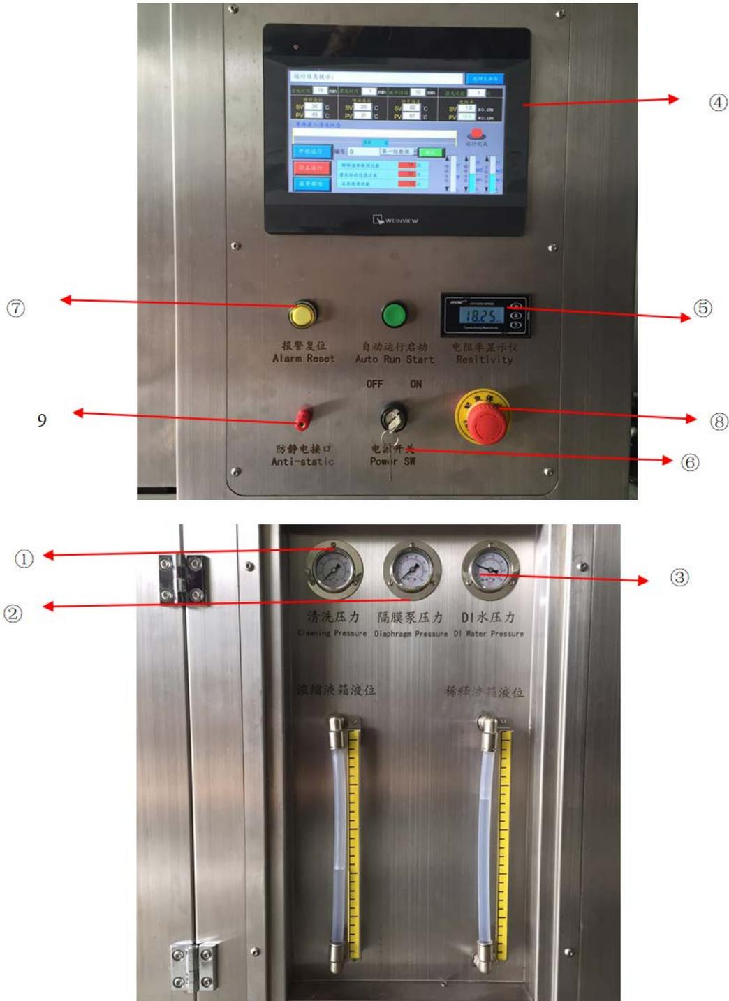
1. Cleaning Liquid pressure: Indicate liquid pressure when it is spraying.
