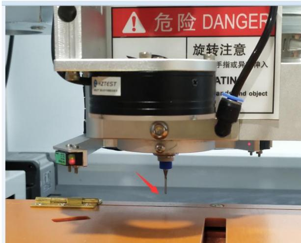
2. After lifting to a safe height, click "Teach" in the position of the cutter head, as shown below;
