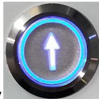
1.6.8 Start the right tray, press this button, the right platform will quickly move to the machine, perform the cutting action.
