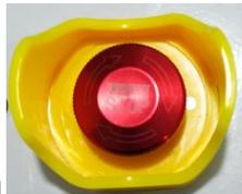
1.6.3 Emergency button , when the machine is abnormal, press this button can emergency stop the machine.
