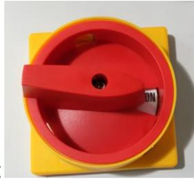
1.6.1 Machine main power: ON: power ON; OFF: power OFF. (When this switch is ON, the industrial computer and the display are energized, but the machine has not been officially started)
