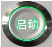
1.6.4 Start button , press this button, the machine can start, which is consistent with the function of the start icon in the software.
