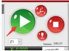
(15) The machine will start, and the tray to be processed is the A/B side shown in the corresponding panorama. Then, press the start button of the left tray and the right tray on the machine panel (**Note: Main (A) is the left platform tray, and Main (B) is the right platform tray**)
