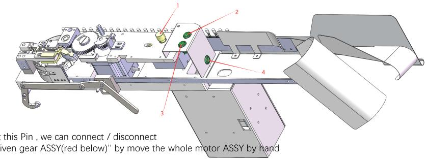
Red mark 1: Motor Pin, with insert / pull out this Pin, we can connect / disconnect between "motor ASSY(green below)" and "driven gear ASSY(red below)" by move the whole motor ASSY by hand
