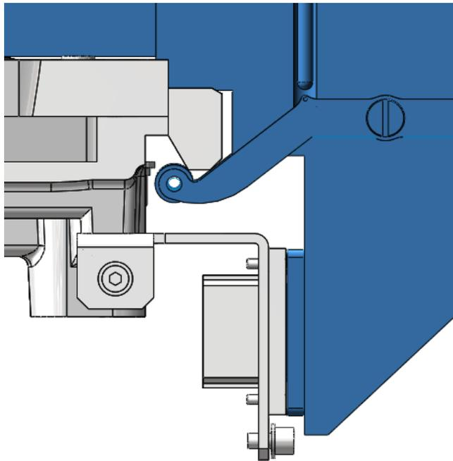
Step 4: release the handlebar and lock in the feeder bank
