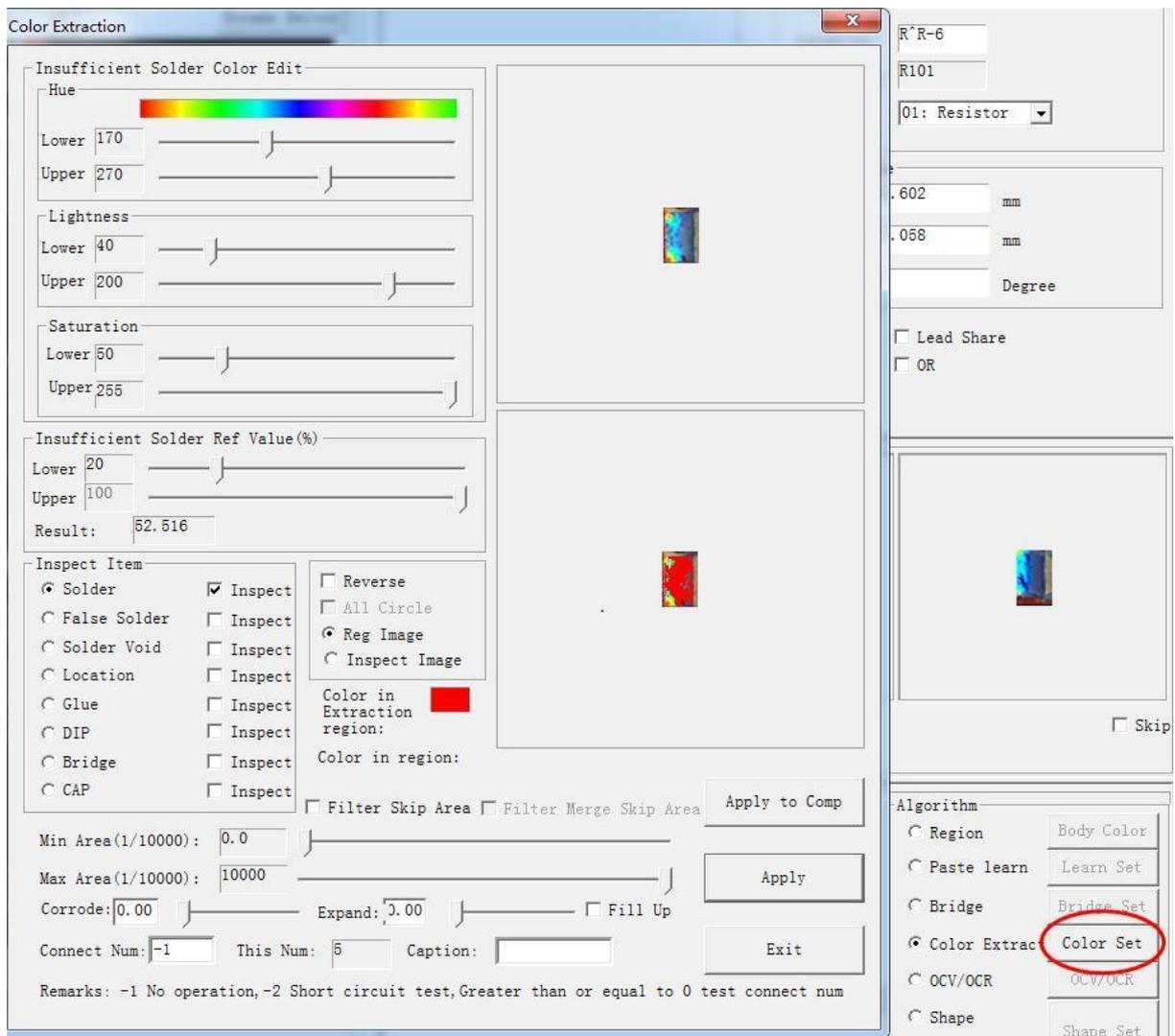
Compared with the single inspection frame of other algorithms which contains only one standard (different standards can be expanded only by adding groups), the single inspection frame for color extraction in this system contains up to 8 different color standards corresponding to color extraction of annular or circular regions, thus increasing flexibility and versatility.
