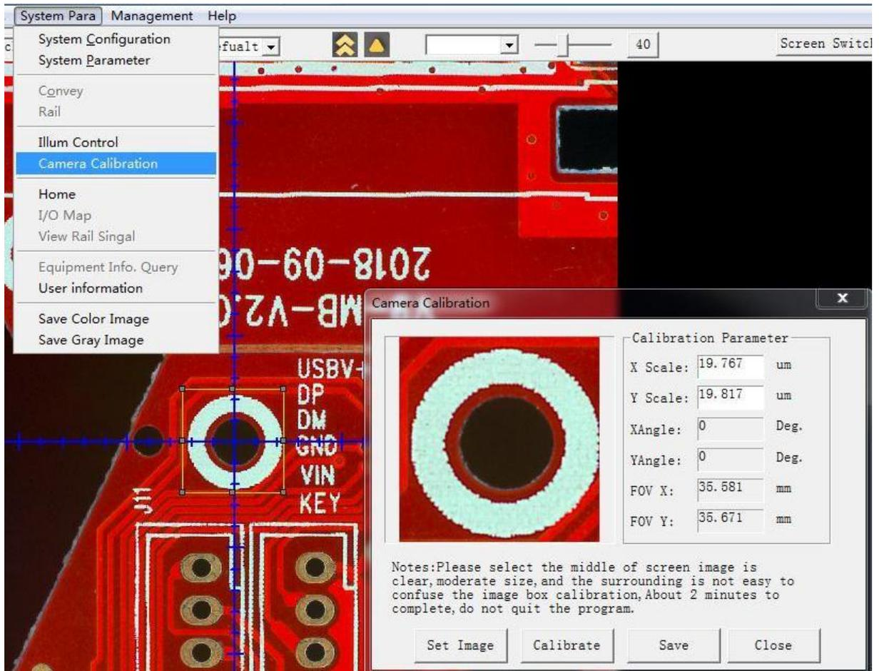
In the editing mode, select the calibration image (preferably circular mark) in the image working area by framing. In this interface, click on the "defining image" button to define the calibration image and press the "starting calibration" button to calibrate. After successful calibration, the calibration
