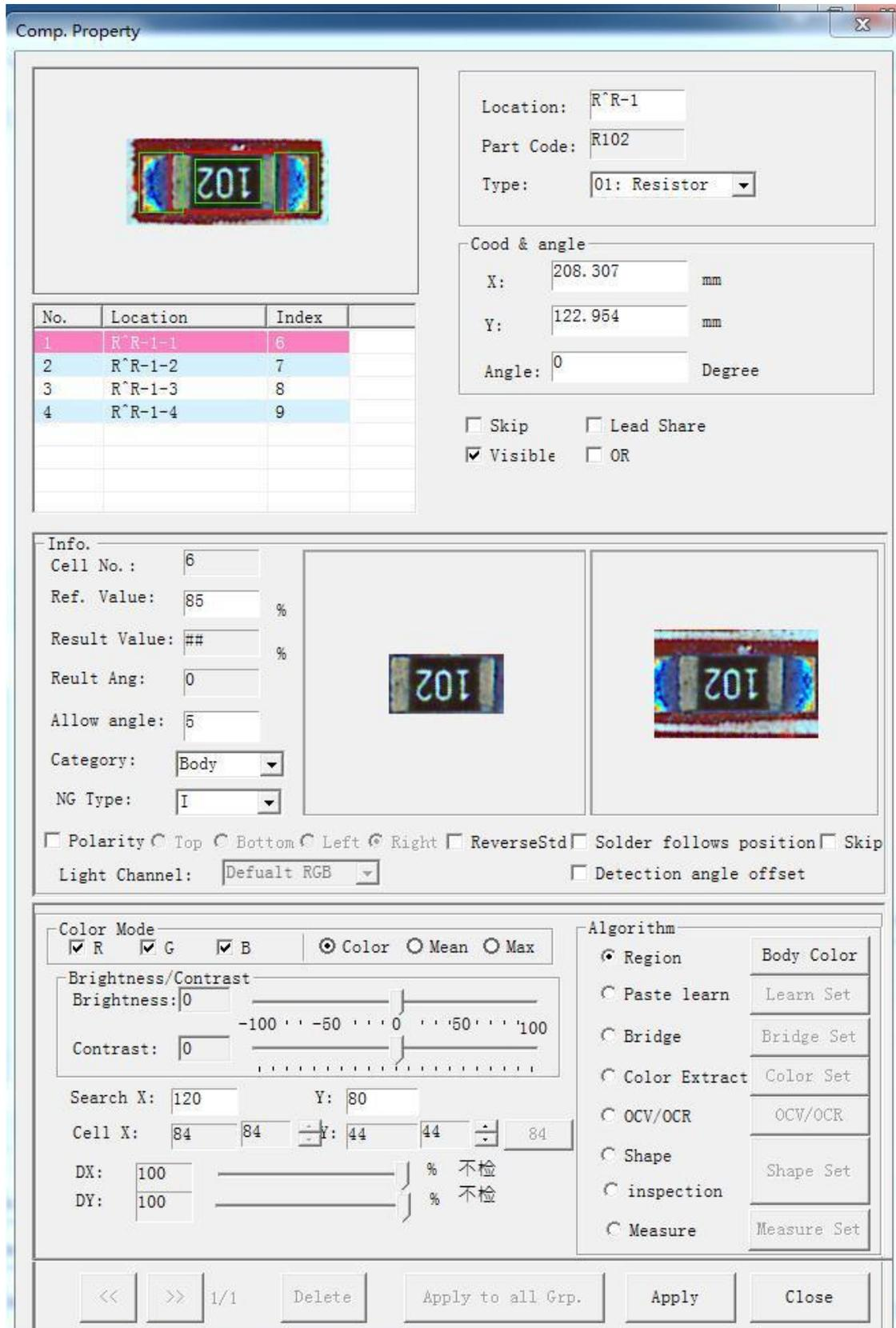
As the container of the inspection frame, the component is a separate hierarchy. The user modifies the component name, shields component inspection, sets whether the component is visible, selects the inspection frame under it and implements other operations in the component attribute window.
