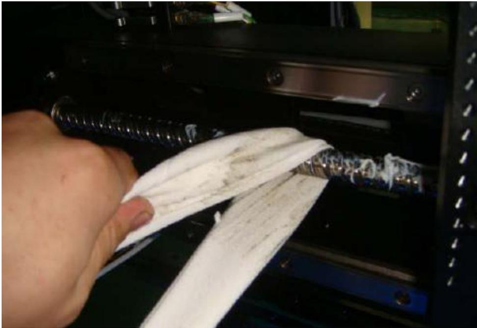
Step 2: apply grease evenly on the surface of the screw rod with a special oil gun, and push the X/Y axis to move back and forth to absorb the grease.
