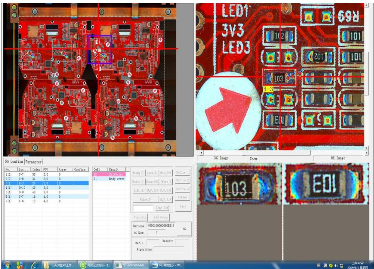
If the current PCB inspection has an inspection frame determined as NG, the NG result display interface will pop up after the inspection is completed for comparison and confirmation by users.
