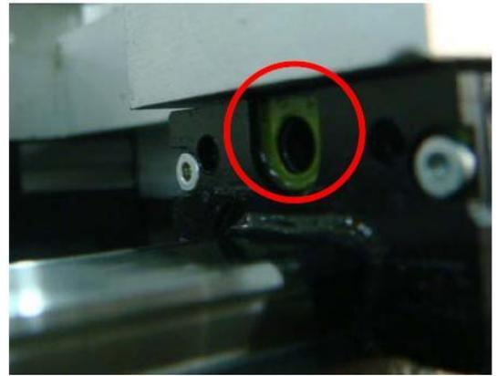
Step 4: insert the oil injection gun head into the oil injection nozzle of the sliding block and press it tightly. Gently press the pressure rod of the oil injection gun to evenly inject grease into the sliding block, and make the sliding block slide back and forth on the guide rail to evenly apply the grease.
